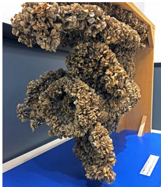
Boat propeller covered with invasive quagga mussels after being submerged in Lake Mead for 11 months.
