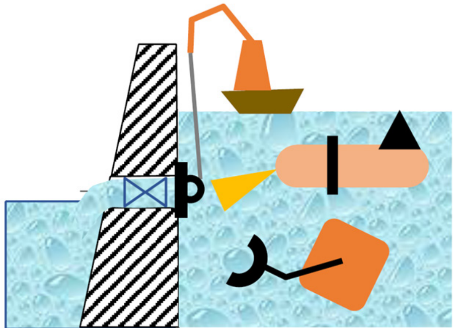
Conceptual engineering solution that applies a sealing plate to the conduit opening using a crane and support from autonomous or remotely operated vehicles as needed.
